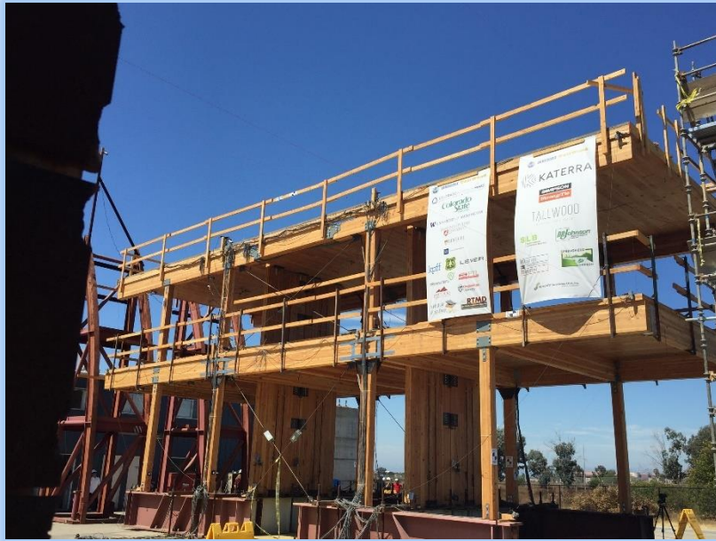
2-Story DRJ CLT & Glulam Beam Structure on a Shake Table in San Diego, CA
