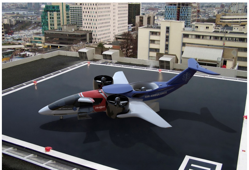
Figure 5 – Conceptual TriFan eVTOL Medevac configuration designed by XTI Corp. for Helijet of Vancouver.
