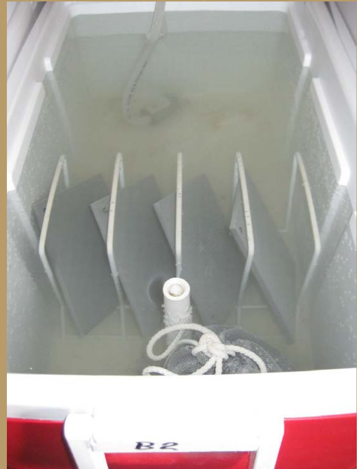
Precipitate observed after 24 hours at pH 9.3
