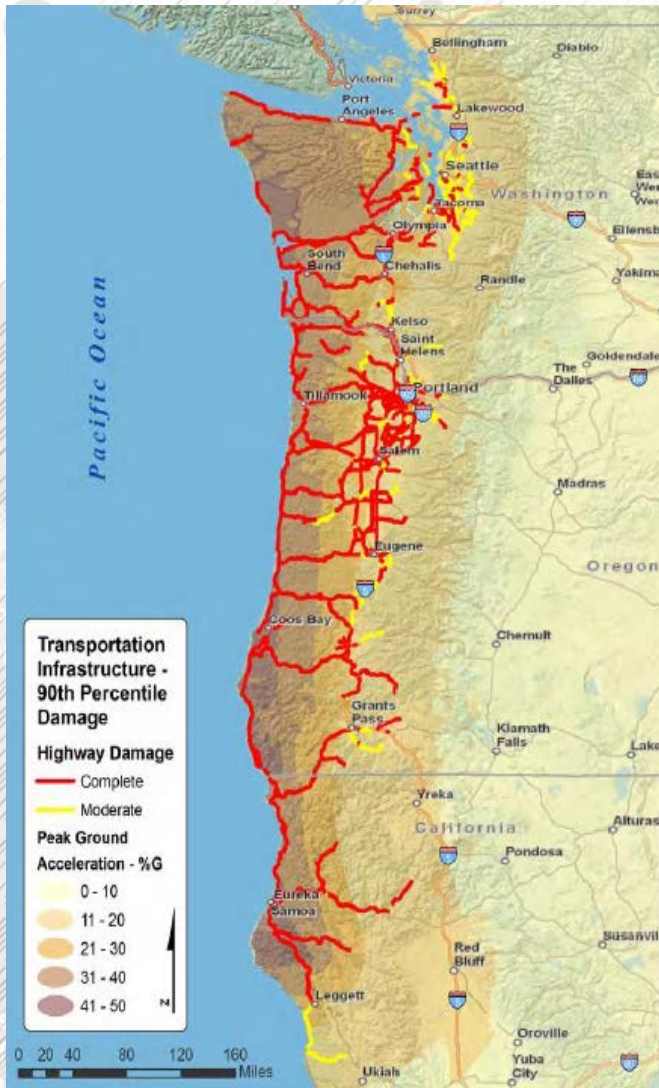
Highway infrastructure estimated damages
